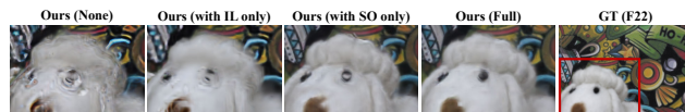
Figure 5. Effectiveness of using in-focus loss and scale optimization for deblur task. IL means in-focus loss, and SO means scale optimization. As we can see, with in-focus loss, color ambiguity caused by defocus blur can be mitigated.
