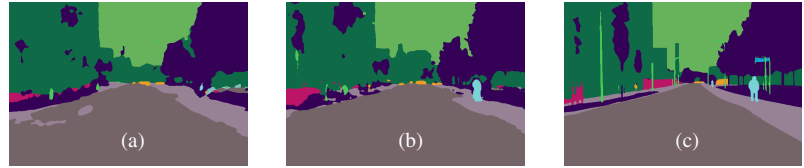
Figure 6. Semantic segmentation on DSEC-Semantic [19]. (a) ViT-from-scratch fails to detect the pedestrian and produces some artifacts on the road. (b) Our MEM rectifies both issues. (c) Ground truth. See Appendix A for more examples.
