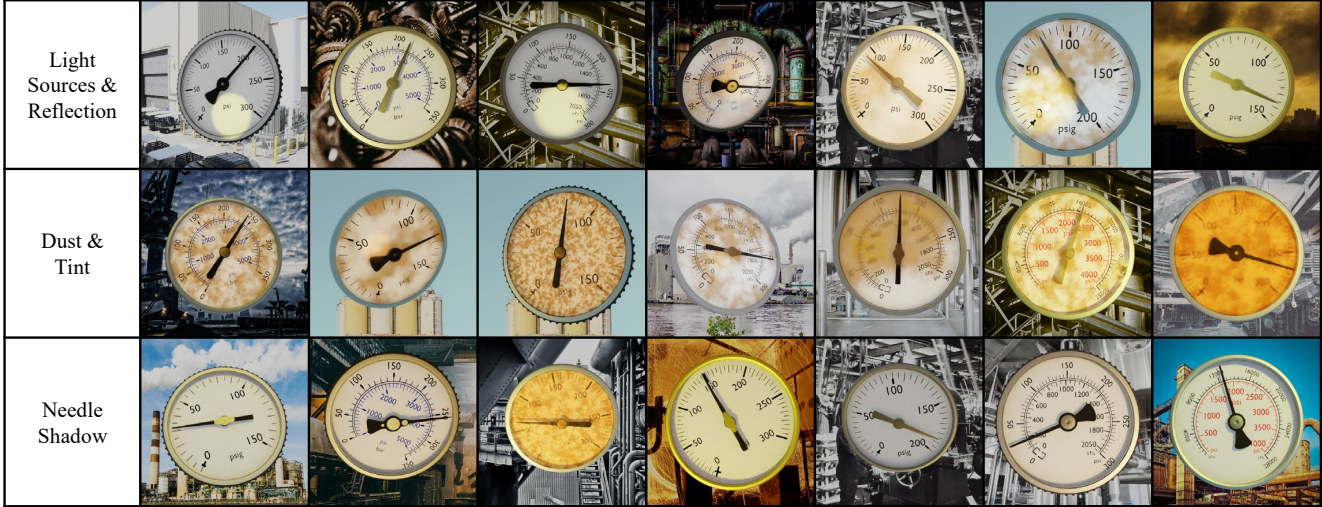
Figure 2. Synthetic Gauge Dataset. We use the 3D creation suite Blender to generate diverse synthetic training samples. We design the rendered samples to include common artifacts and sources of noise, which makes the automatic gauge reading task more challenging. For example, we simulate light reflections on the gauge crystal (first row). We can include different patterns of dust/sand coverage (second row). We also control the needle’s shadow, which can generate alignment errors in the landmark detection task (third row).
