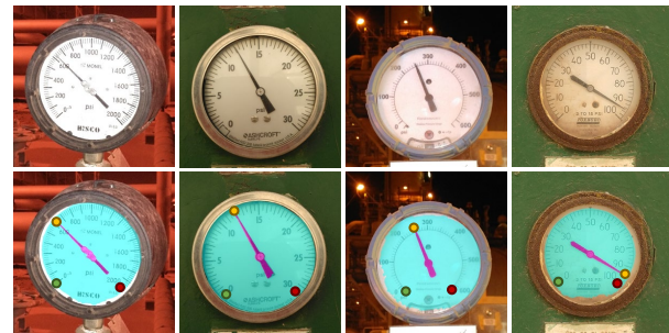
Figure 1. Sample Results. The top row shows samples of gauges captured on the field. The bottom row displays our model's predicted segmentation and regression of landmarks in these images. The segmentation result has three classes: background (not highlighted for easier visualization), gauge (cyan), and needle pointer (magenta). The gauge overlay also contains circles which visualize the estimated locations of the • start marker, • needle pointer, and • end marker.
