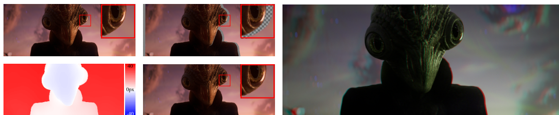
Figure 1. Stereo Conversion. Given a monocular image and a disparity estimate (left), our method performs disparity-aware warping, compositing and inpainting (center) to produce stereo (right, visualized anaglyph). Copyright © 2024 MARVEL. All rights reserved. Permission to use Marvel image only for this publication.
