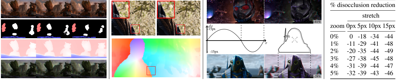
Figure 8. Optional interaction in our approach. Left : Sparse scribbles control the disparity mapping. Center left : Comparison of 2D (left) and 3D (right) movie version with optical flow (bottom). Center right : Implemented mitigation strategies; 15px background stretch, 5% foreground zoom. Right : Reduction of disocclusion areas by mitigation strategies.
