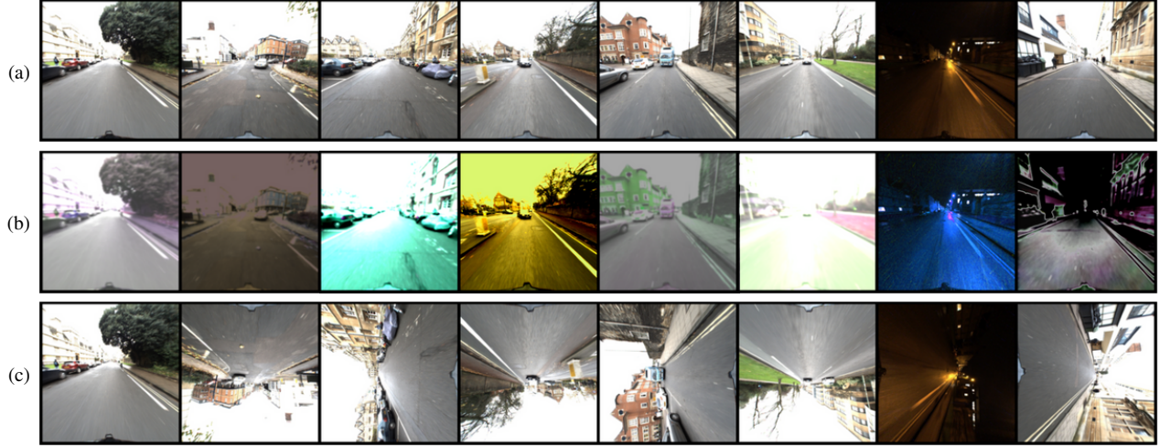
Figure 3. Examples of augmentations leveraged by CLASP-Net. Top row (a): an original input batch from Oxford RobotCar v2 dataset, (b) pixel-level augmentations for appearance changes, (c) examples of rotations applied to the original image.
