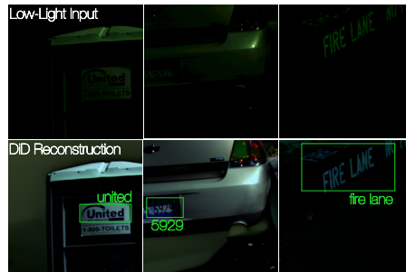
Figure 7. DiD reconstructs unseen, real low-light data. Results from running PARSeq [7] on SID Sony low-light data [10]. Green signifies correct text recognition. Low-light inputs are scaled for visualization.
