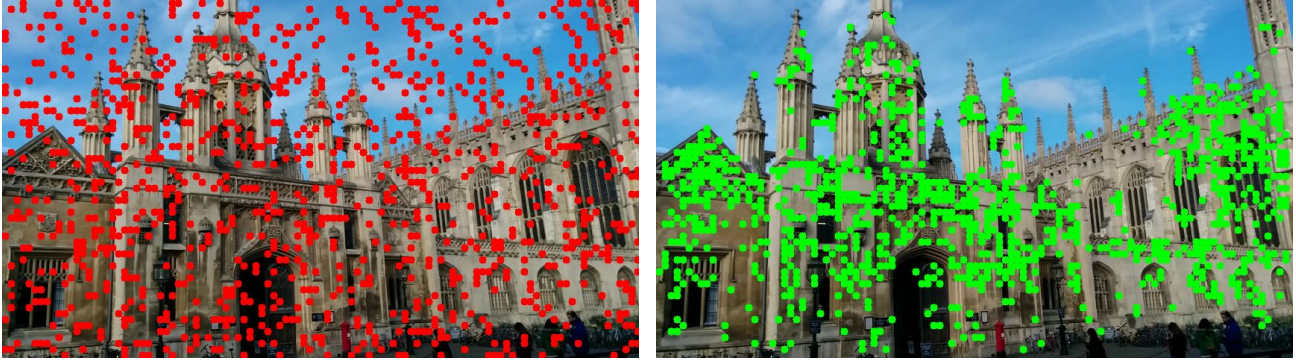
Figure 4. Sampling strategies comparison. (Left image) An example of the sampled pixels (red dots) using random sampling. (Right image) An example of the sampled pixels (green dots) using our sampler. Our sampler focuses on important building structures instead of unimportant, texture-less regions (e.g., the sky) of the image.
