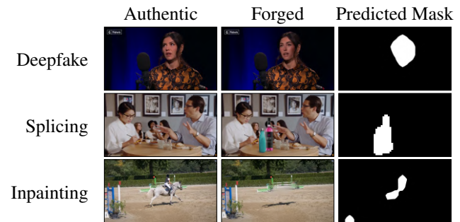
Figure 1. Sample video forgery localization results obtained using our proposed VideoFACT network on videos modified by deepfaking (Top), splicing in an object (Middle), and removing an object with inpainting (Bottom).
