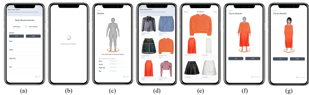
Figure 7. The pipeline of a prototype for applying ViBA-Net in a real application. Step (a): inputting the personal information; step (b): generating a 3D SMPL model according to the input measurements data; step (c): adjusting and confirming the body shape; step (d): browsing the fashion items; step (e): selecting one favour clothing item with corresponding outfit recommendations that consider the body shape; step (f): visualizing the outfit composition on the size of body shape; step (g): translating the SMPL model into a human image via generative model e.g., Midjourney.
