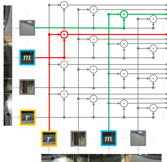
Figure 4. Illustration of the self-attention mechanism of transformer. Whereas the red colored dot product denotes the high attention between m \in \mathcal{M} and r \in \mathcal{R} , the green colored dot product denotes low attention between m \in \mathcal{M} and a certain token in single layer image regions outside of \mathcal{R} .
