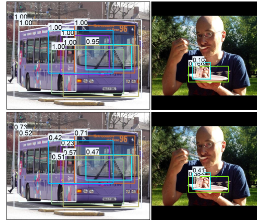
Figure 1. Comparison of box predictions for novel classes ‘bus’ and ‘cake’ between ViLD [10] (top) and our approach (bottom). Low-quality boxes have similar scores to high-quality ones, leading to high false positive (left) and false negative rates (right) in ViLD while being eliminated in our LP-OVOD.
