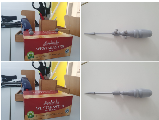
Figure 3. Real images of the tea box and a texture-less tool with markers (top) and their inpainted counterparts where markers were removed (bottom). This example suggests that our marker removal process does not differentiate between rendered and real images.
