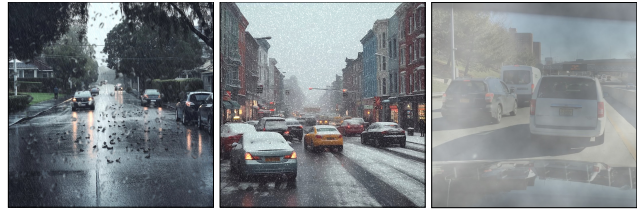
Figure 3. Images from the dataset with image corruptions. The left image showcases synthetic rain-streaks and raindrops. The middle image displays a synthetic snow overlay. The right image shows a clear image transformed with the synthetic fog model.
