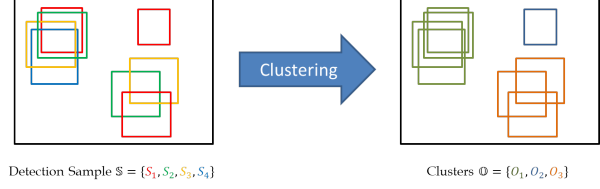
Figure 2. An illustration of image clustering based on predictions obtained from F = 4 forward passes, with |S_1| = 3 , |S_2| = 2 , |S_3| = 2 , and |S_4| = 1 . The aim is to group predicted instances that correspond to the same object into distinct clusters \mathbb{O} . In this example, |O_1| = 4 , |O_2| = 1 , and |O_3| = 3 , where each cluster O_m \mid m \in \{1, 2, 3\} represents an instance.
