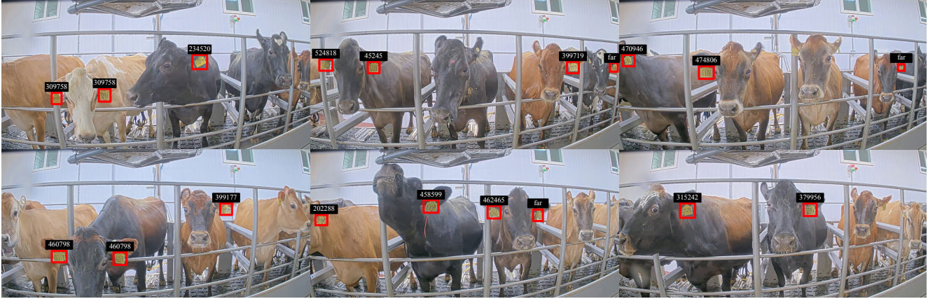
Figure 4. Example output frames from ReadMyCow system operating in real dairy farm. The bounding box line thickness and size of the text predictions have been enlarged for visibility.
