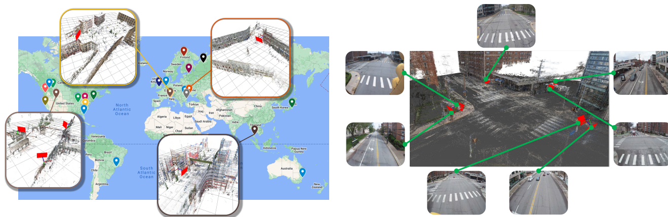
Figure 1. Our framework allows us to perform 3D scene reconstruction and precise localization of over 100 real-world traffic cameras distributed globally across multiple countries, with the potential to scale to any camera with sufficient street-level imagery. (Left) : Highlighting the reconstruction and localization of traffic cameras at specific chosen locations. (Right) : Demonstrating 7 cameras positioned within an urban intersection, accurately localized with respect to the reconstructed 3D scene. Please zoom in for better visualization.
