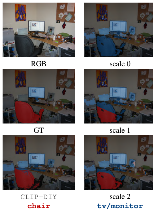
Figure 5. Qualitative ablation study. In the right column we show the results when progressively adding more scales in the multi-scale approach. Running with 3 scales enables segmenting most of the chair.
