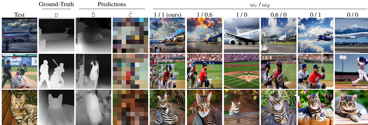
Figure 8. Effect of the Composition Weight in GIR (Sec. 4.3). The two weights \omega_c and \omega_d control the relative importance of corresponding features from three deciphered cues: semantics, color, and depth. When predicted depth or color fail to provide reliable guidance, we can manually tweak the weights to achieve satisfactory reconstructed results.
