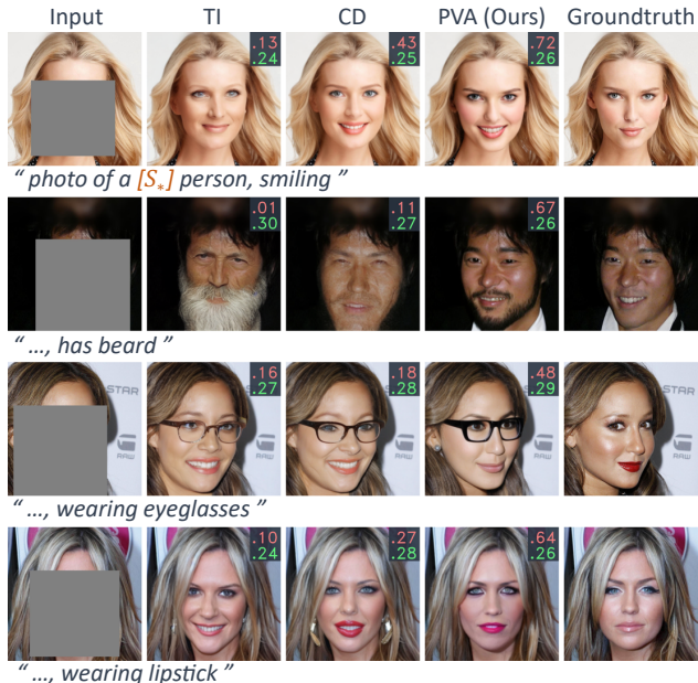
Figure 4. Qualitative comparisons of identity-preserving language-controlled inpainting. Prompts for editing are shown at the bottom of each row. We annotate the ID similarity (line 1) to the groundtruth and the CLIP similarity (line 2) to the text prompt at the upper right of each inpainted image.
