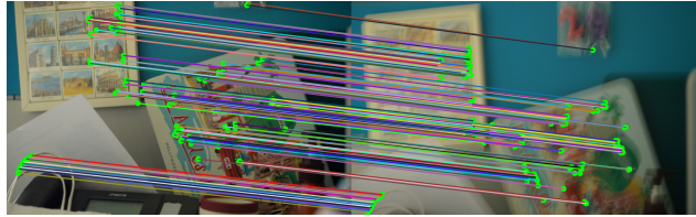
Figure 5. Qualitative evaluations on real blurred image. The experimental results demonstrate that our network is able to detect well distributed and localized keypoints from either sharp and blurred images for further image matching.
