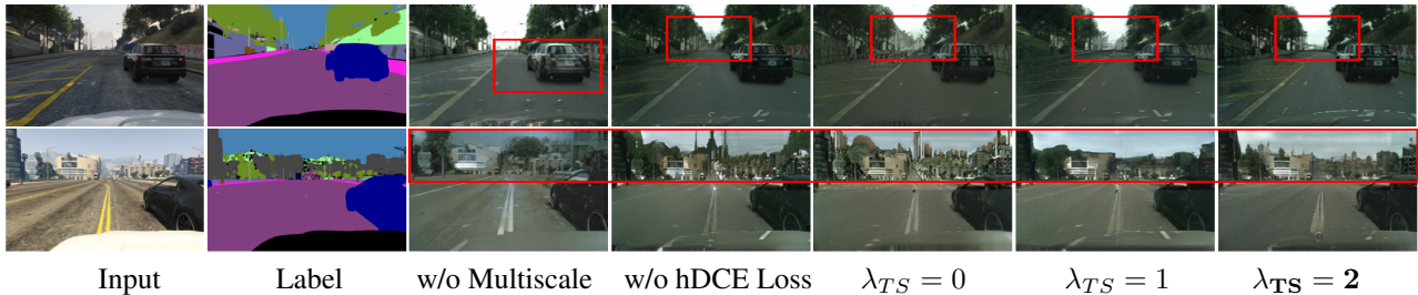
Figure 7. Qualitative ablation study for GTA5 to Cityscapes. The red bounding boxes indicate artifacts. Removing multi-scale prediction yields inaccurate predictions and blurry results. Eliminating either the hDCE or TS loss introduces more artifacts and semantic distortion. As the weight of TS loss increases, semantic distortion is reduced.
