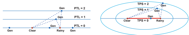
Figure 4: Comparing Point To Line (PTL) with Triangular Probability Similarity (TPS): PTL employs unconstrained optimization, pushing the generated image ‘Gen’ onto the straight line connecting ‘Clear’ and ‘Rainy’, frequently ends up on the extension cords. In contrast, TPS uses constrained optimization, adjusting the ellipse level set to position the generated image on the line segment connecting ‘Clear’ and ‘Rainy’. Zoom in for better view.
