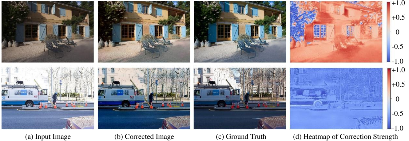
Figure 4. Heatmap of Correction Strength in our MSLT. (a) the under/over exposed input images. (b) the corrected images by our MSLT. (c) the “ground truth” images. (d) the heatmaps of correction strength described in §3.3. The values in (0, 1] (or [-1, 0) ) indicate brightness enhancement (or shrinkage). Darker color indicates larger absolute values and stronger correction strength in brightness.
