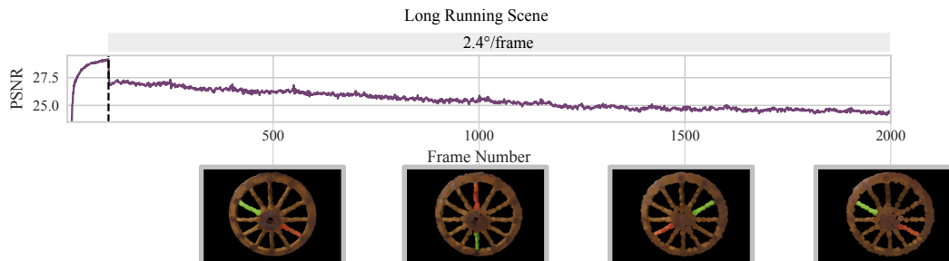
Supplementary Figure 5. Figure showing degradation that occurs over a longer sequence of the Wheel dataset. The initial loss in quality is because the transition from static to 2.4 degrees is more sudden than the static to 1.2 degrees used in earlier experiments. Degradation occurs as particles begin to lose neighbours and are unable to acquire new ones.
