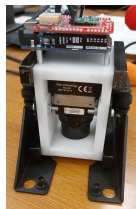
Figure 7. The aerial pod used for mounting the thermal camera on the light airplane's underbelly.
