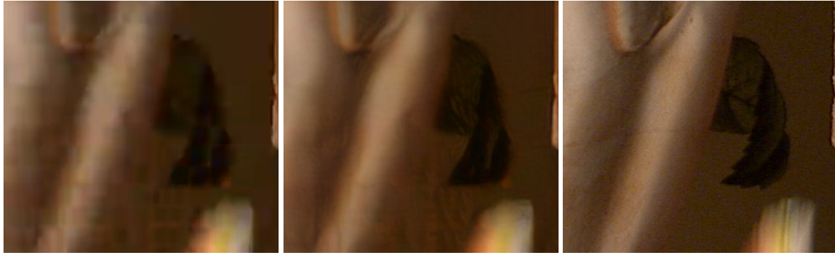
Figure 7. Compression Artifacts Mistaken for Texture. Crop from 1920 \times 1080 “Cactus”. The compressed image exhibits strong chroma subsampling artifacts (lower right corner). These are mistaken by the GAN as a texture and restored as such.
