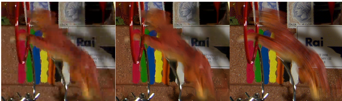
Figure 8. Motion Blur. Crop from 1920 \times 1080 “Cactus”. The tiger exhibits high motion which presents itself in the target frame as motion blur. This blur is destroyed by compression and is not able to be restored by the GAN loss. The GAN loss is also “rewarded” for sharp edges which would make reconstructing blurry objects difficult. As an aside, note the additional detail on the background objects in the GAN image when compared to the compressed image.
