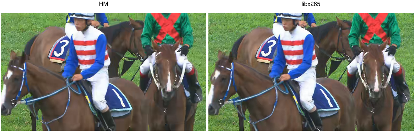
Figure 2. Codec Comparison. HM reference encoder vs. libx265 at QP37. While the artifacts produced by the different encoders are different, the overall perceptual quality is similar. This is likely because of CQP encoding which does not leave many options for the encoder to make intelligent rate-distortion decisions.
