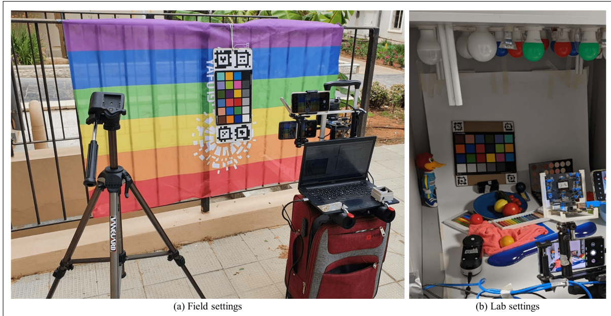
Figure S2. Beyond RGB dataset collection: (a) Capturing outdoor scene, with the color-chart presented using MS sensor and 2 Android devices. (b) Automated scene capturing in lab viewing booth, with the color-chart presented, using MS sensor and 2 Android devices, and an automated spectrophotometer measurement. Notice the various light sources present in the custom viewing booth.
