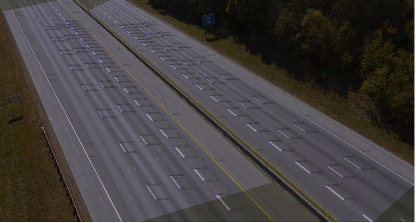
Figure 1. Correspondence points (blue) and fields of view (shaded polygons) for each roadway direction of travel, labeled in a single camera field of view (P27C01). Around 100 correspondence points are visible for each side of the roadway.
