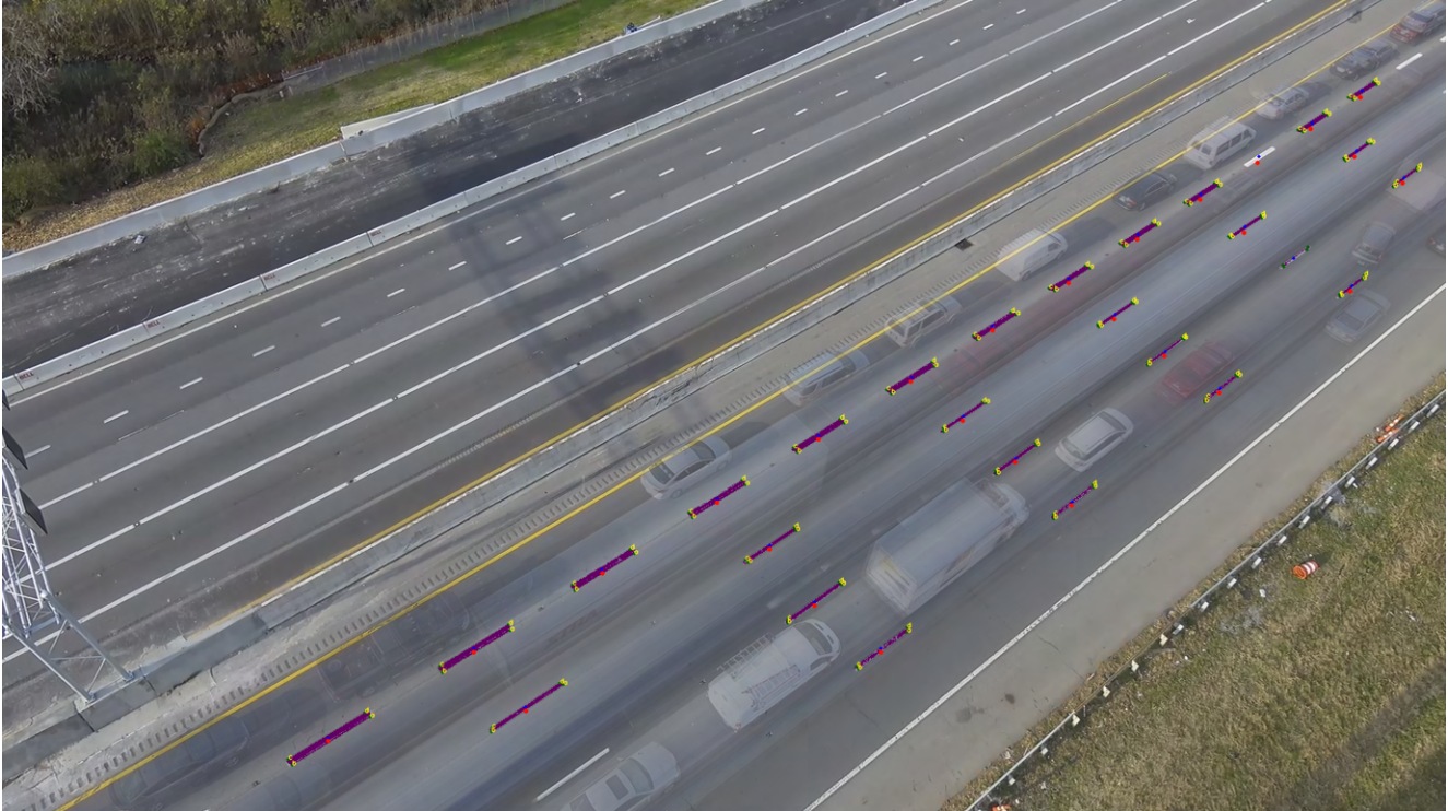
Figure 7. An example of SIFT-FLANN based seed points from step 6 (red dots), detected contours (purple outlines) and re-detected dash corner points (yellow dots) for a 1-minute average frame. Because traffic at this time instance was partially stopped, some vehicle artifacts are visible in the averaged frame. A few dashes are not successfully rediscovered.
