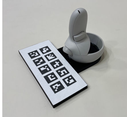
Figure 10. Calibration tool used to align coordinate frames between the RGB camera and the Meta Quest 2 headset. The controller is rigidly connected to the ArUco board.
