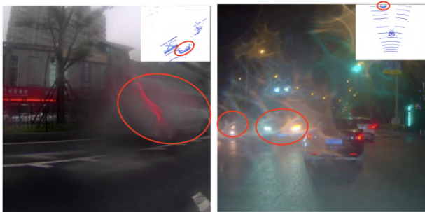
Figure 1. Example of retrieval using separate prompts for image and lidar. We query for images with blur, water spray, glare, corruption, and lack of objects, and for point clouds with nearby trucks, pedestrians, cars, etc. By combining the scores of these separate queries, we can find edge cases that are extremely valuable during the training/validation of a camera-based perception system. These valuable objects are highlighted in red, both in the image and point cloud.
