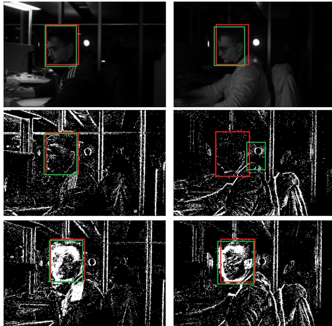
Figure 14. Face detection on three samples (Indoor, with an incandescent bulb). Left is GS data, right is IR. The first row is APS, others are EVS. The first two rows show a static face, while the third row shows a moving face. Ground truths are in red, predictions in green. Notice the different event density around the face when there is a movement, vs. when there is none.
