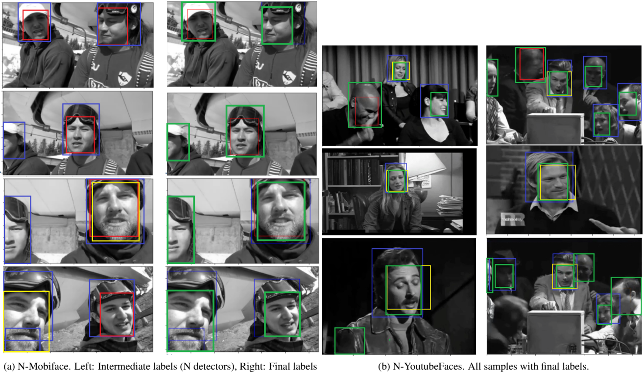
Figure 7. Illustration of the pseudo-labeling process, before and after the Non-Maximum Suppression (NMS). Red boxes: MTCNN, Blue boxes: Yolov5, Yellow boxes: Initial ground truth, Green boxes: Final label after NMS. Best viewed in color.
