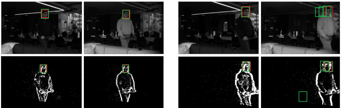
Figure 15. Face detection on two samples from N-SpectralFace (Indoor with sunlight). For each group of pictures, the first row is APS GS and APS IR, and the second row is EVS GS and EVS IR. Ground truths are in red, predictions in green. Notice how the single channel IR models show more false positives.
