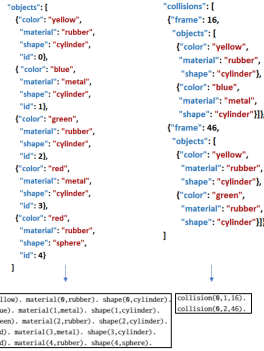
Figure 9. Conversion of improved object detection (video frame parser) results into ASP facts.
