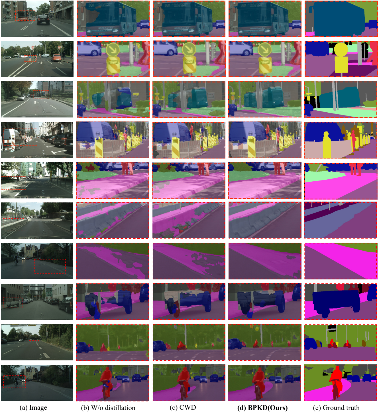
Figure 4. Qualitative results on the Cityscapes [1] validation set produced by PSPNet [11] and ResNet18 network architecture: (a) Initial images, (b) w/o distillation, (c) state-of-the-art method channel-wise distillation [7], (d) BPKD our method, (e) Ground truth. This figure shows that our methods segment the small complex objects with explicit boundaries. Zoom in for a better view. In the first row, BPKD effectively addresses the issue of the front windshield of the bus being wrongly segmented into multiple classes. In the second row, the approach enhances the contours of the upper and lower sections of the road signs. The third row presents a particularly striking result in the segmentation of a train; through differentiated supervision and distillation of the edges and main body, the train is clearly segregated from obstructions. In the fourth row, distant pedestrians present a challenging case for segmentation and identification due to their far-off camera angle and significant occlusions; despite these complexities, BPKD still manages to produce stable edges around the human figures. In the remaining images, BPKD consistently shows improvements, achieving commendable segmentation outcomes on both pedestrian paths and roadways.
