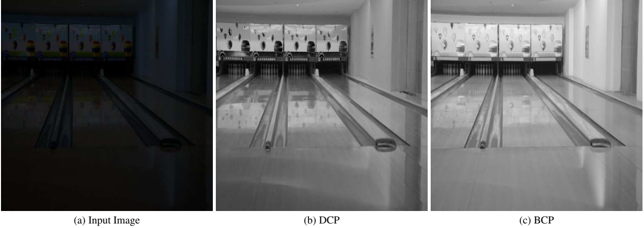
Figure S.1. (a) Input low-light image, (b) dark channel prior (DCP) for low-light image, (c) bright channel prior (BCP) for the low-light image.
