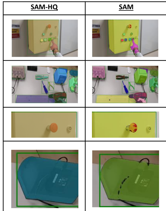
Figure 6. Comparison between SAM-HQ (left) and standard SAM (right). We reported also the bounding boxes (in green) used to generate segmentation masks.
