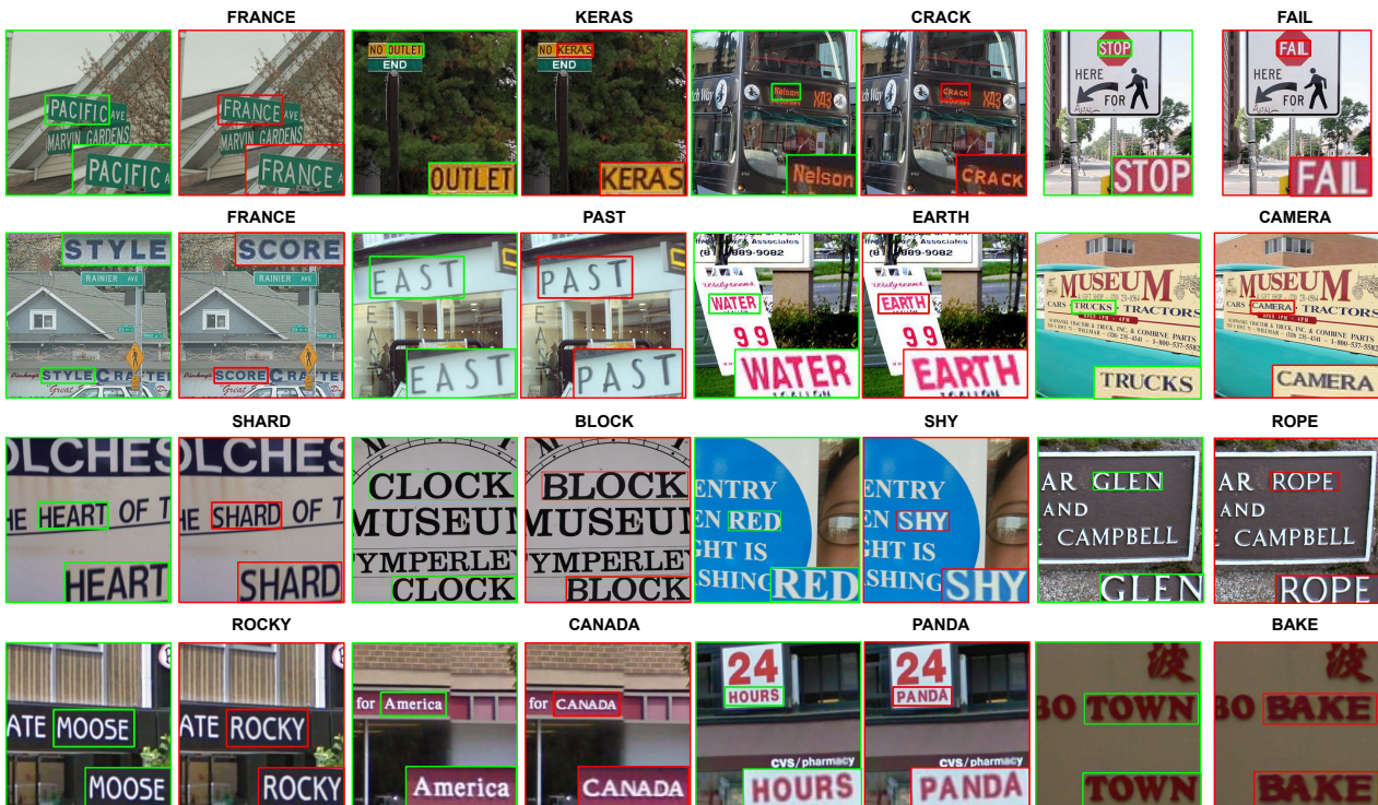
Figure 3. Given a cropped single word from in-the-wild images using a bounding box marked by a green box , and specifying the desired text, our method successfully edits the text to match the desired text and can replace the original word in the original image, as shown by red box .
