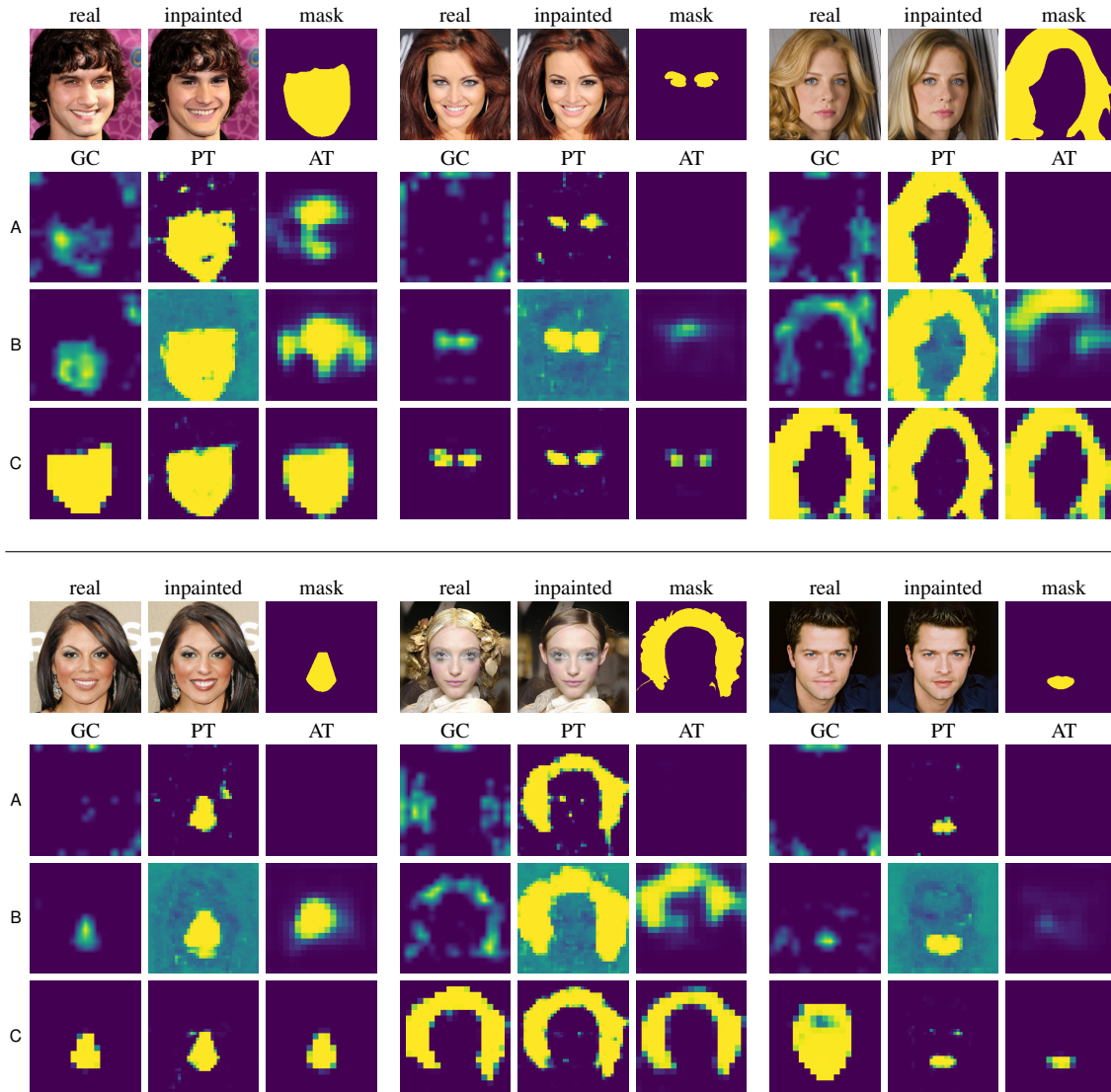
Figure 1. Soft localization maps produced by the three proposed approaches using different level of supervision. Patches can accurately detect the manipulations after having seen only fully generated fake images (scenario A) or locally-inpainted images with only image-level supervision (scenario B). Both Attention and GradCam struggle in scenarios A and B. All methods recover the manipulated region in the fully supervised scenario, C. This suggests that operating at a patch level is better suited for recovering local manipulations than either using a GradCam or Attention.
