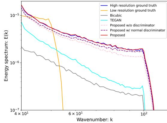
Figure 11. The velocity energy spectra of a van case
