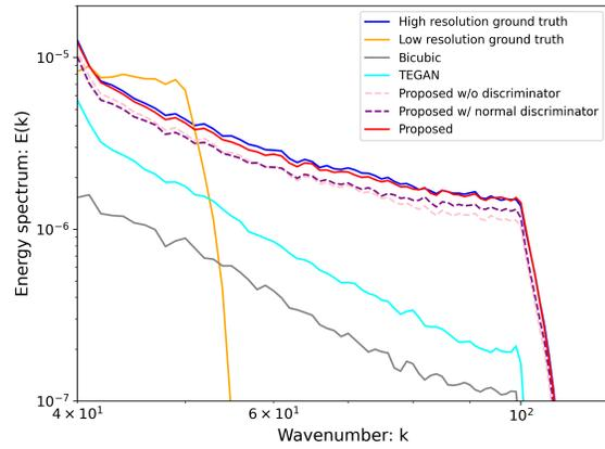
Figure 13. The velocity energy spectra of a small car case
