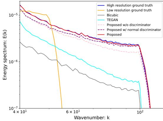
Figure 10. The velocity energy spectra of a pickup truck case
