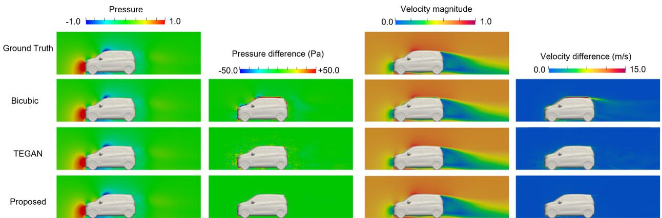
Figure 5. Differences comparison on a small car case
