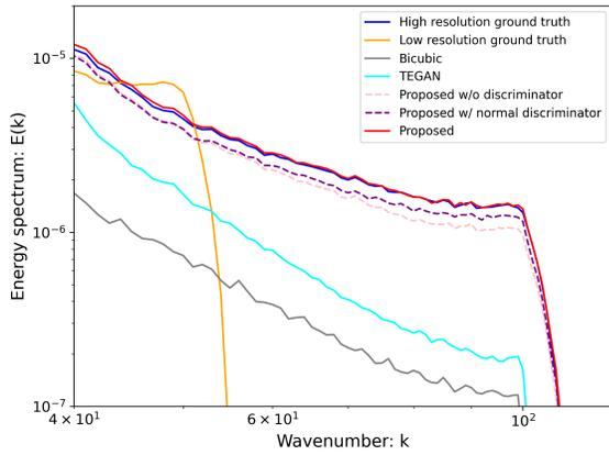
Figure 12. The velocity energy spectra of a sedan case
