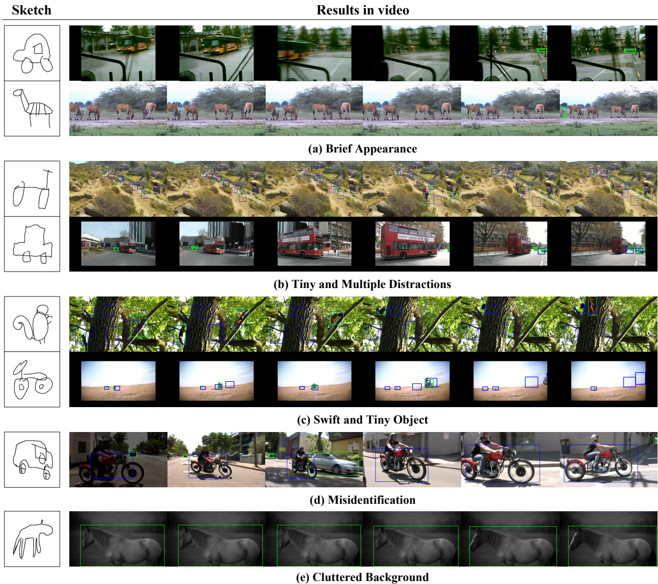
Figure 7. Failure cases of SVANet on QuickDraw dataset. Green and blue boxes represent ground truths and predictions, respectively.
