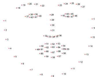
Figure 1. The positions for the 68 facial landmarks. Image is adapted from the iBUG 300-W dataset [9].
