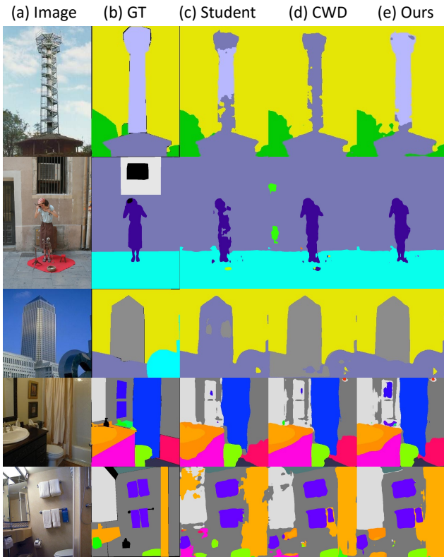
Figure 1. Qualitative segmentation results on the validation set of ADE20K using the PSPNet-ResNet18 network: (a) raw images, (b) ground truth, (c) student, (d) channel wise distillation, (e) our method FAKD.
