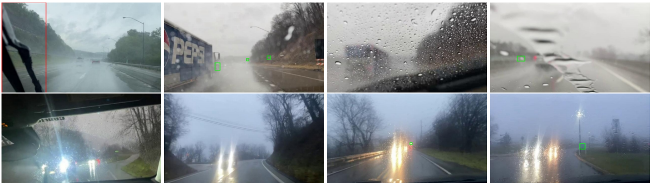
Figure 5: Failure cases for the proposed method. Red: Yolov3 pretrained on clear weather images. Green: Yolov3 finetuned on our generated rainy images.
