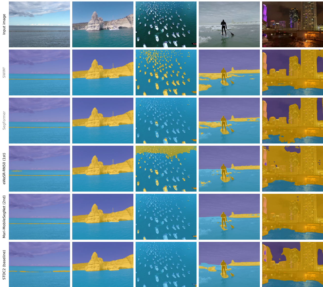
Figure 9: Qualitative comparison of methods for USV-based embedded obstacle segmentation.
