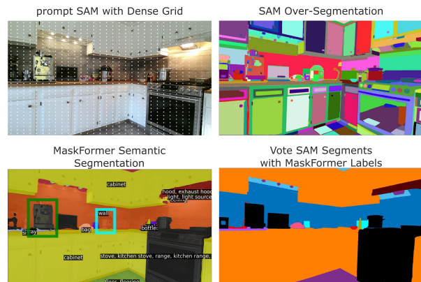
Figure 3. An example of labeling using Semantic Segmentation (MaskFormer) and SAM. MaskFormer produces good predictions for foreground classes but not so well for foreground classes: the coffee machine is misclassified as a ‘stove’ (black bounding box), and the cooking pot (cyan bounding box) is missed entirely.
