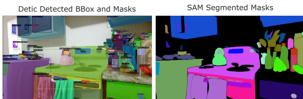
Figure 4. An example of labeling using Object Detector (Detic) and SAM.
