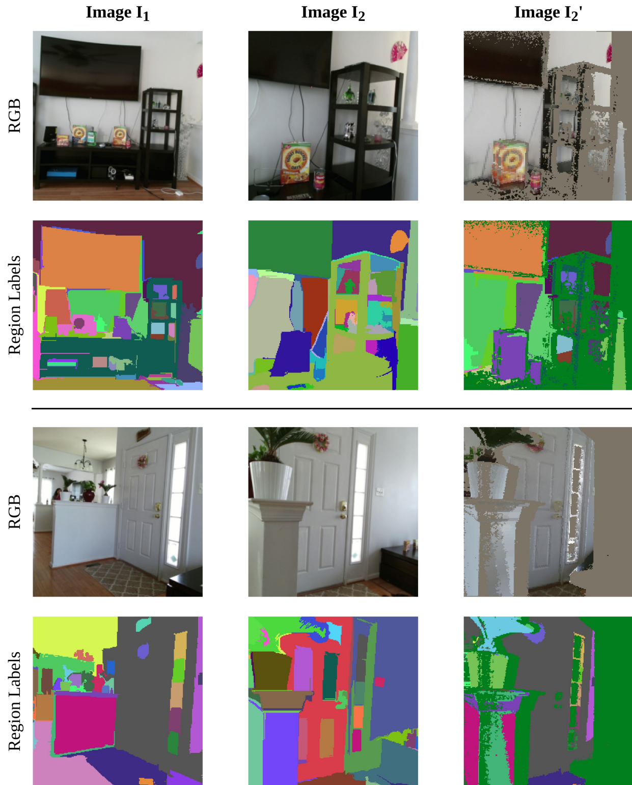
Figure 4. Examples of projection from I_1 to I_2 resulting in I_2' inside AVD scene. Some pixels in I_2' are invalid because of occlusion and missing or erroneous depth. Such pixels share the same label and color in the visualization in I_2' and are not used during pre-training.
