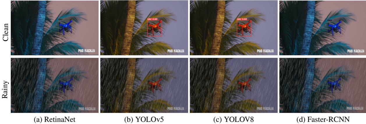
Figure 5. Comparisons on clean TS images and rainy RTS images. RetinaNet and Faster-RCNN detect the UAV in the rainy image with lower confidence; however, YOLOv5 and YOLOv8 do not detect the UAV in the rainy image (best viewed on screen when zoomed-in).
