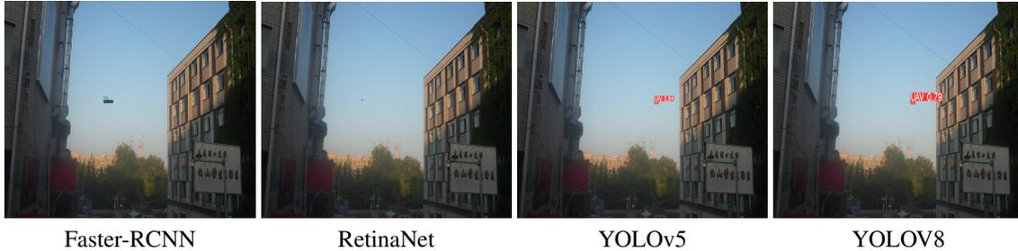
Figure 7. Sample detection outputs: Faster-RCNN, Yolov8, and YOLOv5 detect the UAV; however, RetinaNet fails to detect the UAV.
