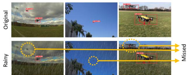
Figure 1. Rain artifacts degrade the performance of a state-of-the-art model for UAV detection; bottom-row shows the missed UAVs and low-confidence detections of the model due to rain artifacts. These vividly highlight the adverse effects of weather and complex backgrounds on UAV detection accuracy, highlighting the implications of rain-induced distortions and artifacts for detection and localization models in real-world surveillance.
