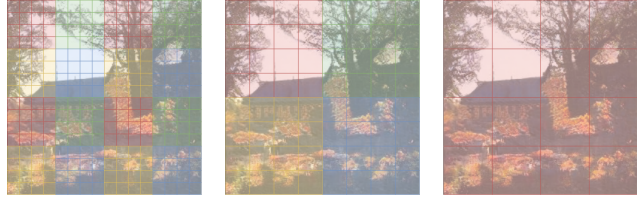
Figure 1. Attention matrices of a Swin transformer at different resolutions. Each grid cell represents a token, while colored regions correspond to the attention regions. The number of attention regions is reduced as cell grids are linearly combined during pooling. The size of attention regions remains constant.
