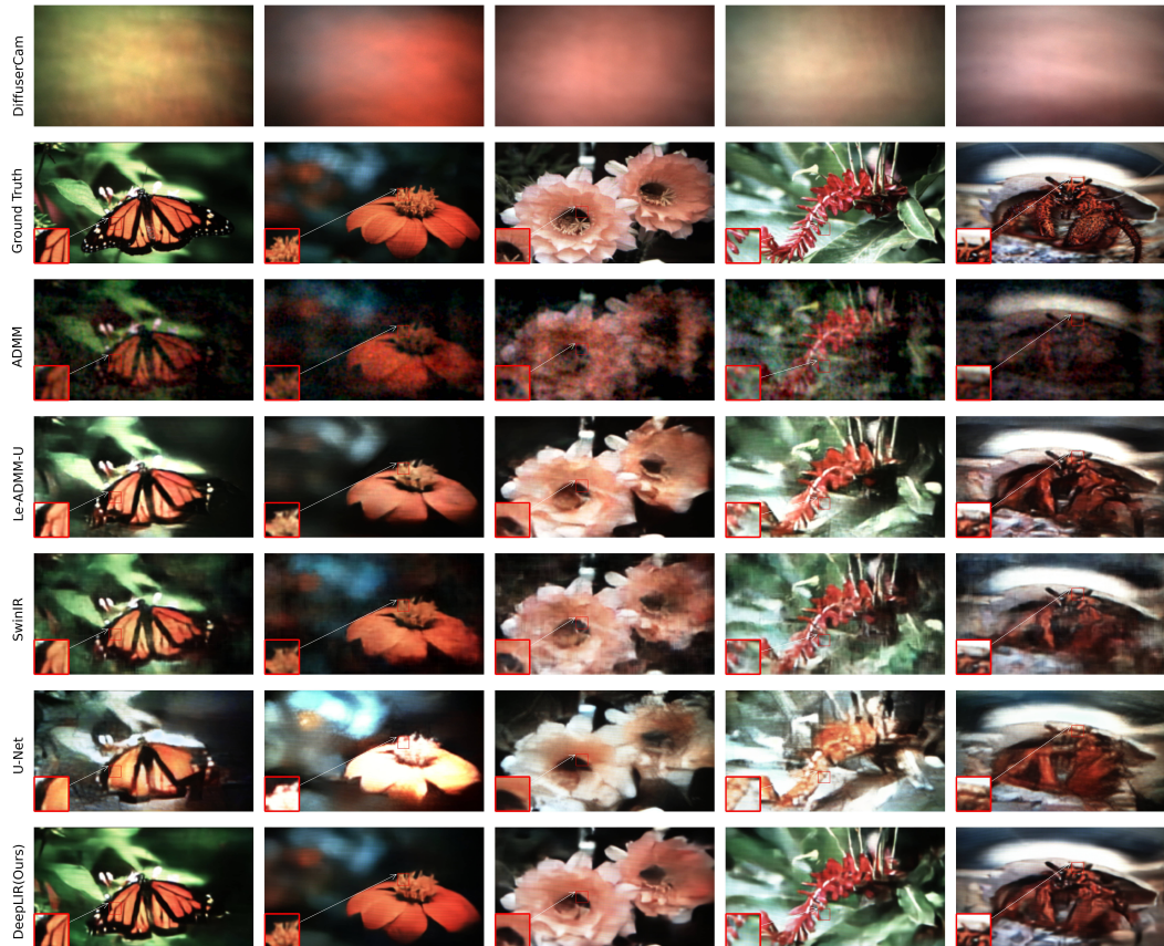
Figure 4. Comparative image reconstructions from DiffuserCam measurements using various models. Big red box: Zoom in version of the indicated smaller red box. DeepLIR is able to reconstruct complex patterns and fine details where other models fail. You may zoom in to view more details.
