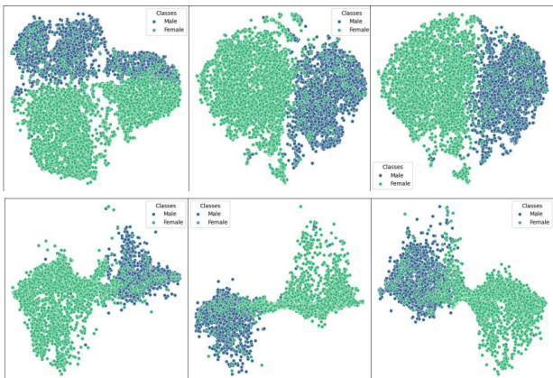
Figure 5. t-SNE plots feature representations for models (first row: BEiT and second row: ResNet-50) trained on real and synthetic datasets across different perturbations, from left: Blockwise Distortion (BW), Color Contrast (CC), and Color Saturation (CS).
