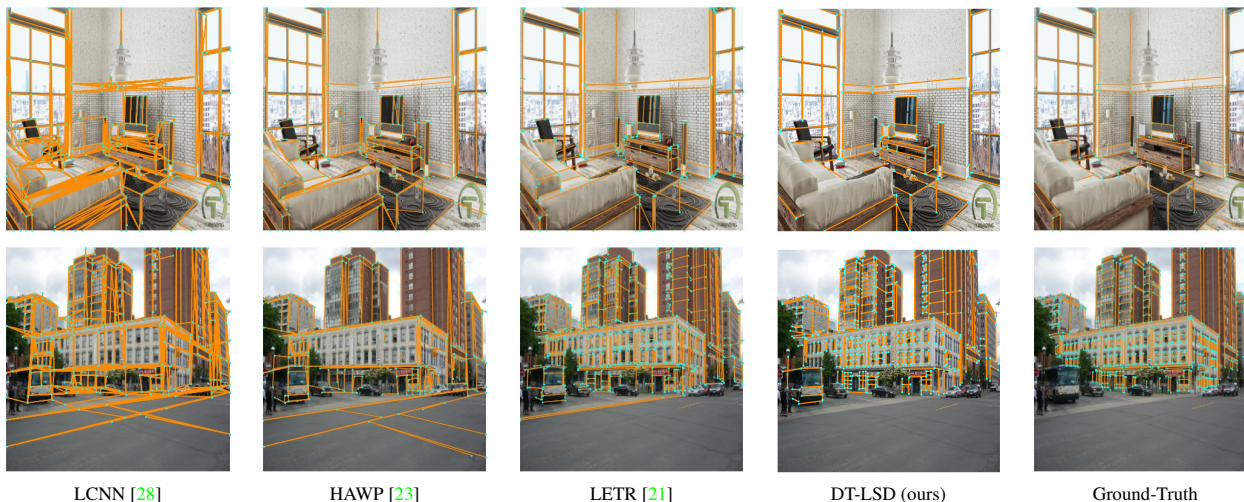
Figure 6. Qualitative comparisons for line detection methods. From left to right: the columns provide example results from LCNN, HAWP, LETR, DT-LSD (ours) and the ground-truth. The top and bottom rows provide examples from the Wireframe and YorkUrban test sets, respectively. The bottom two rows provide examples from the YorkUrban test set.
